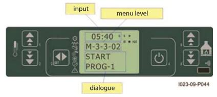
The weekly programmer consists of 4 independent programmes which can be combined together in different ways. The weekly programmer can be enabled or disabled.
