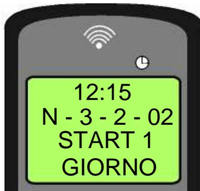
It is possible to set two on/off times defined by the times set according to the table below. If the value is set to OFF, the time clock ignores the control.
