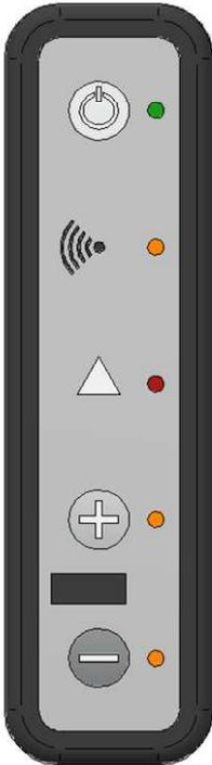
ON/OFF button: to manually switch the stove on or off
