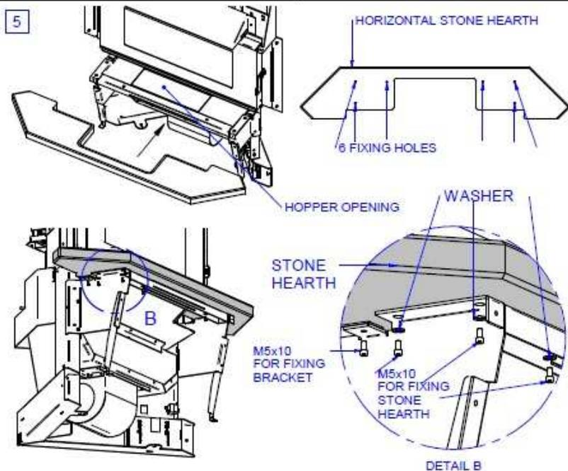
INSERT STONE HEARTH CENTERING IT WITH RESPECT TO HOPPER OPENING AND FIX IT INTO PLACE USING THE SIX M5x10 SCREWS.
