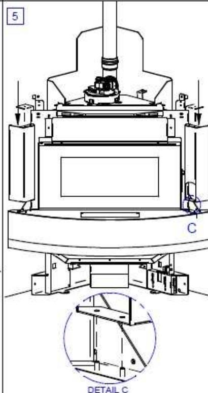
INSERT THE TWO SIDE COLUMNS MAKING SURE THAT HOLES CORRESPOND TO THE TWO LOWER CASING SCREWS
