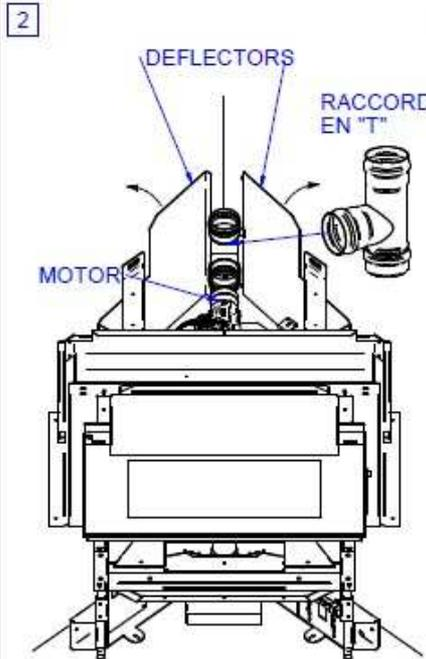
OPEN DEFLECTORS TO INSERT TEE (NOT SUPPLIED) IN EXHAUST MOTOR MORE EASILY.
