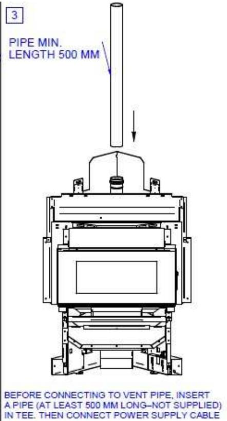
BEFORE CONNECTING TO VENT PIPE, INSERT A PIPE (AT LEAST 500 MM LONG - NOT SUPPLIED) IN TEE. THEN CONNECT POWER SUPPLY CABLE
