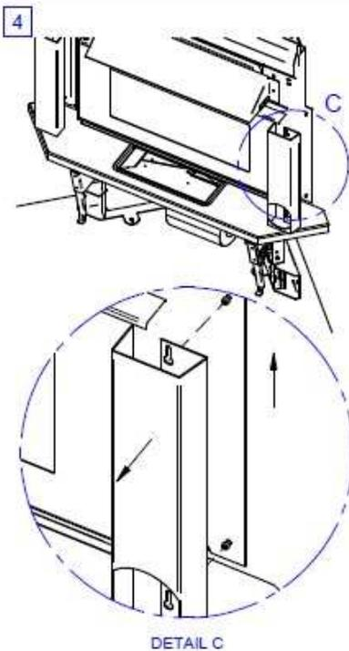
REMOVE THE TWO SIDE COLUMNS BY PULLING THEM UPWARDS
