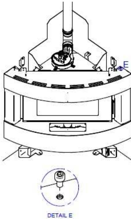
FIX UPPER CASING USING THE TWO M6x10 SCREWS
