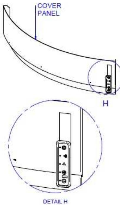
ATTACH ADHESIVE DISPLAY ON RELEVANT SEAT IN COVER PANEL
