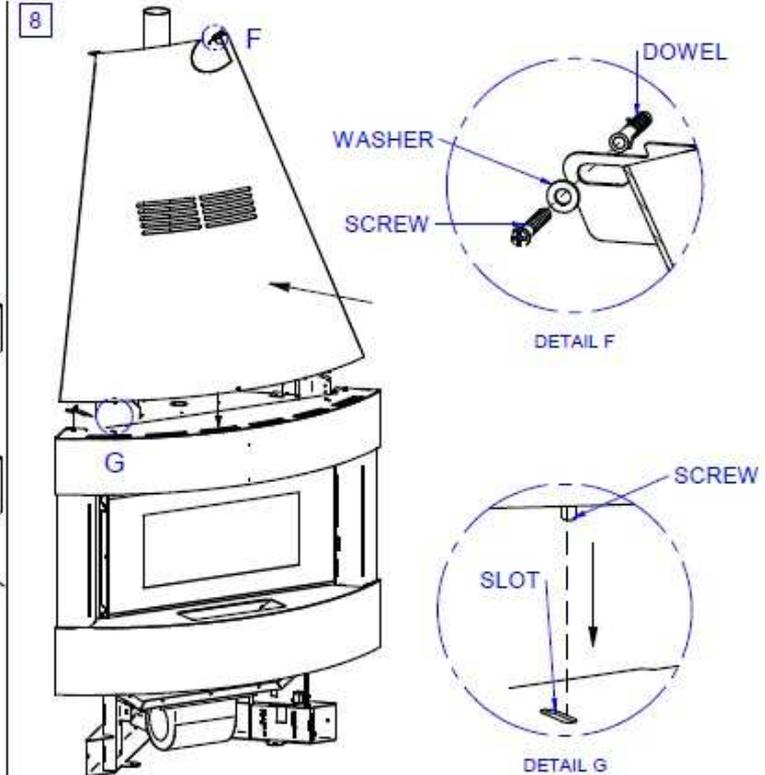
INSERT HOOD MAKING SURE THAT THE TWO SCREWS CORRESPOND TO UPPER CASING SLOTS
