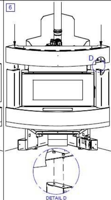
INSERT UPPER CASING MAKING SURE THAT SCREWS CORRESPOND TO SIDE COLUMN HOLES
