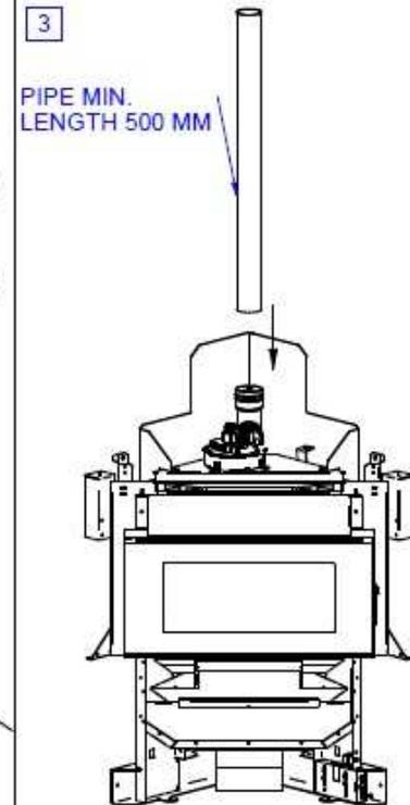
BEFORE CONNECTING TO VENT PIPE, INSERT A PIPE (AT LEAST 500 MM-LONG) IN TEE. THEN CONNECT POWER SUPPLY CABLE.
