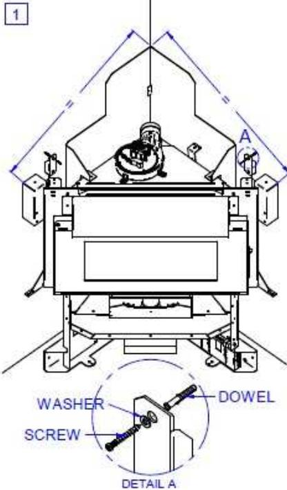
MAKE SURE THAT DISTANCE BETWEEN BRACKET AND WALL CORNER IS THE SAME ON BOTH SIDES. FIX STRUCTURE USING SCREWS AND DOWELS (Ø 6).
