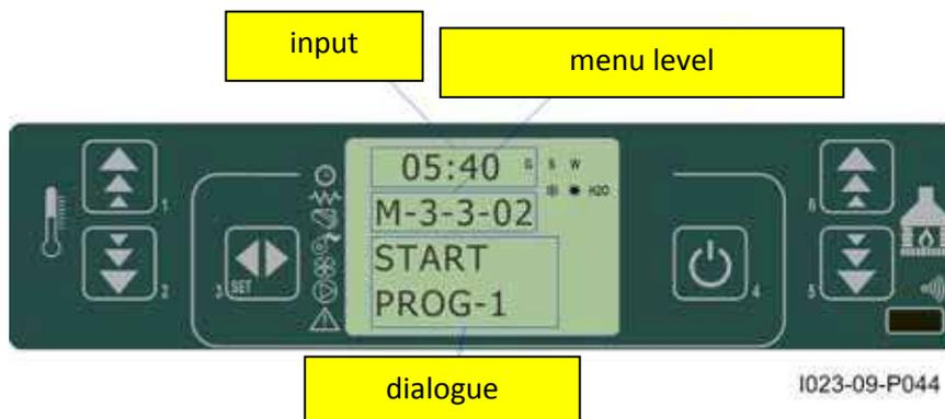
The weekly programmer consists of 4 independent programmes which can be combined together in different ways.
