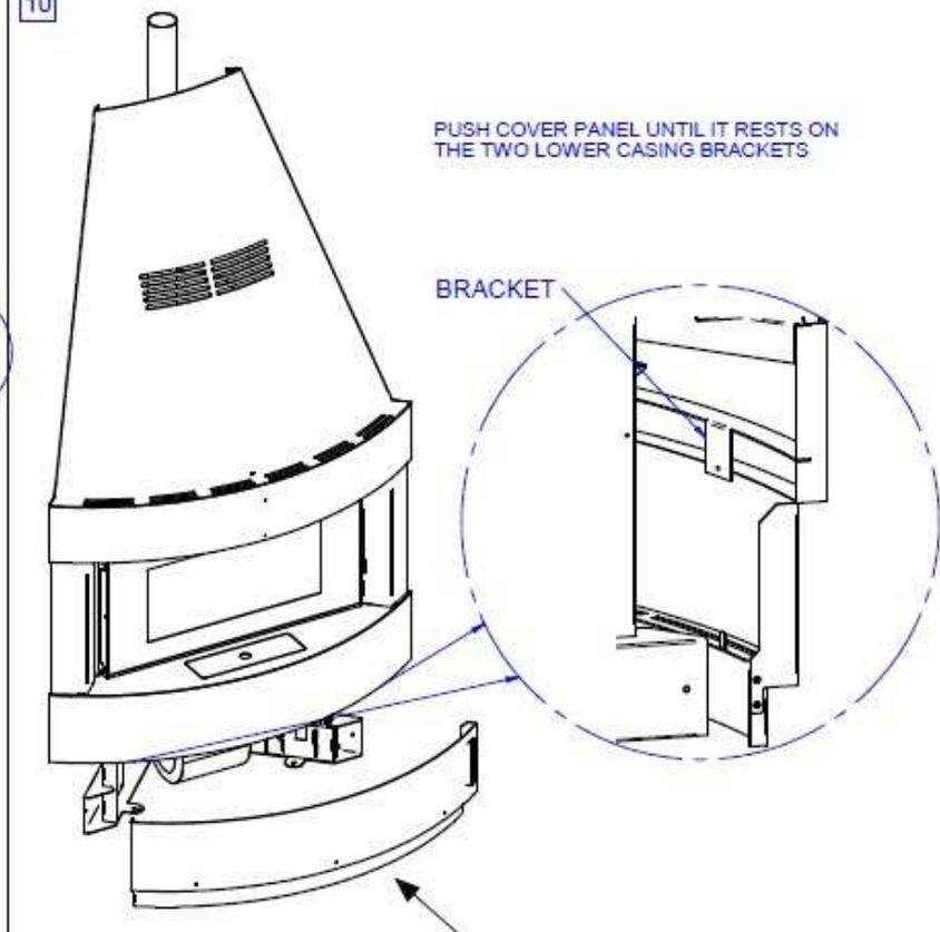
PUSH COVER PANEL UNTIL IT RESTS ON THE TWO LOWER CASING BRACKETS
