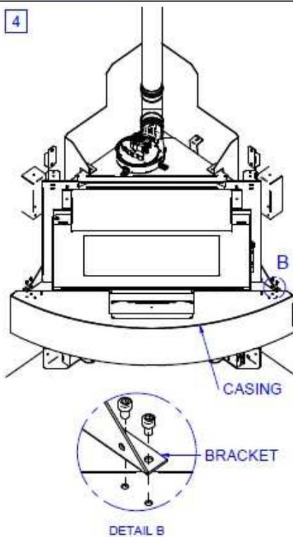
FIX LOWER CASING TO INSERT BRACKETS USING THE FOUR M8x10 SCREWS
