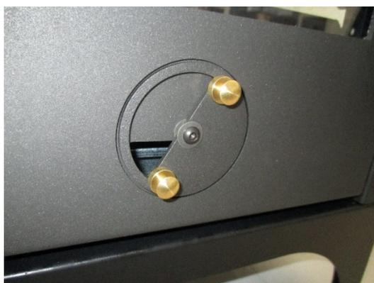
When refilling with wood it would be advisable to open the secondary air adjustment device (NOT THE PRIMARY ONE). Slightly open the door so that the stove takes in oxygen, load the wood and close the firebox door. At the time of refilling there should be no lit fire in the chamber as, depending on the efficiency of the fireplace, there may be a loss of fumes into the environment generated by the fire. Therefore, refilling is only recommended when there are embers burning on the fire bed.
