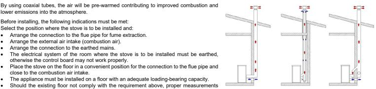
must be taken (for instance, the installation of a load distribution plate). All the structures which could catch fire if exposed to excessive heat must be protected. Floors made from wood or inflammable materials must be protected using non-combustible materials (e.g. 4mm-thick sheet metal or ceramic glass).
