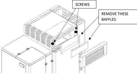
Then reposition the finned front panel.
